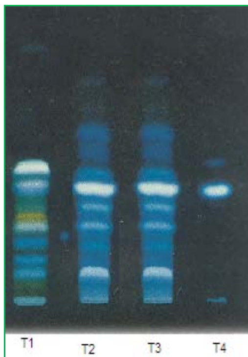
Figure 1f: TLC fingerprint profile of Ferula foetida Track 1: Ferula foetida ; Track 2: Sulaharana Yoga (Sharmayu); Track 3: Sulaharana Yoga (In-house); Track 4: Umbelliferone ; Solvent System: Toluene: ether (1:1 saturated with 10% acetic acid)
